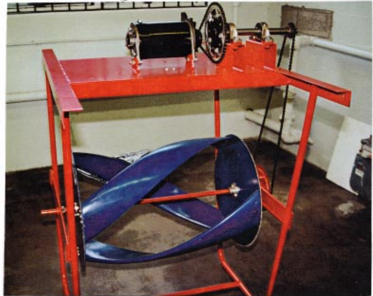
Triple-Helix Turbine (generator above water)
